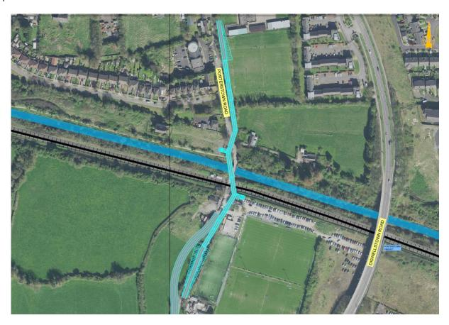
Figure 3-74 Porterstown Option 3 – Pedestrian and Cycle Bridge – Straight Approach Ramp (Copyright Ordnance Survey Ireland – 0039720)
