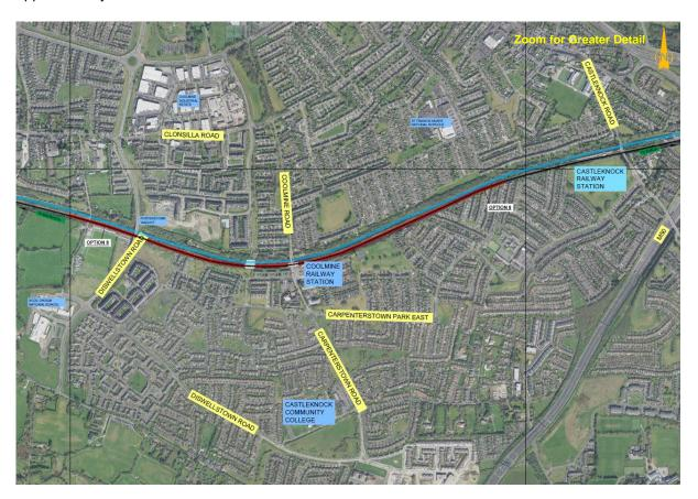
Figure 3-68 Coolmine option 8 - lowering of the railway vertical alignment (Copyright Ordnance Survey Ireland – 0039720)
