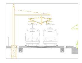
Figure 3-7 Single Track Cantilever cross section
