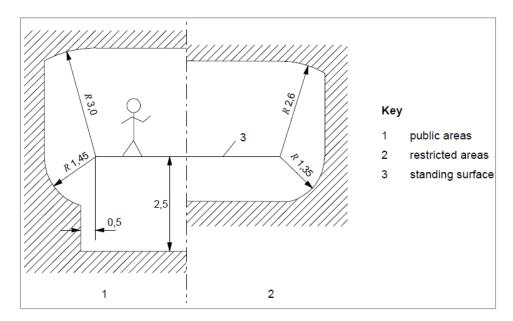
Figure 3-11 Minimum clearances to live parts outside vehicles and to live parts of OHLE from standing surfaces
