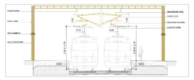
Figure 3-10 Proposed DART+ West OHLE structure in stations
