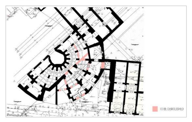
Figure 3-130 Rotunda Building Structural Modifications Requirements
