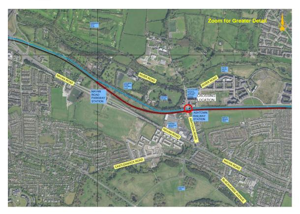
Figure 3-43 Ashtown Option 9 - Lowering of the Railway Vertical Alignment (Copyright Ordnance Survey Ireland – 0039720)
