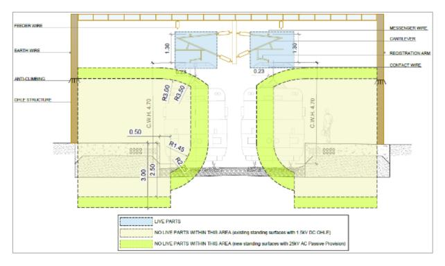
Figure 3-12 Portal in Stations for DART+ West: Protection against direct contact (25kV AC Passive Provision is not applicable to DART+ West)
