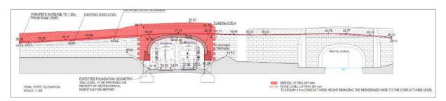
Figure 3-28 Deck reconstruction of the OBG11: precast arch deck solution
