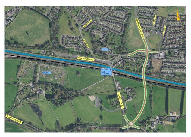
Figure 3-84 Clonsilla Option 7 - Overbridge 200 metres to the east - online of Larchgrove with retaining walls (Copyright Ordnance Survey Ireland - 0039720)
