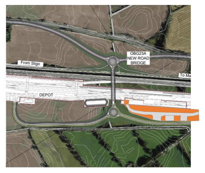
Figure 3-175 Depot Access Option 4 (Focus on Access)
