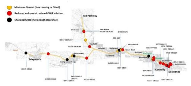
Figure 3-26 Overbridges with less than 'Enhanced' clearance
